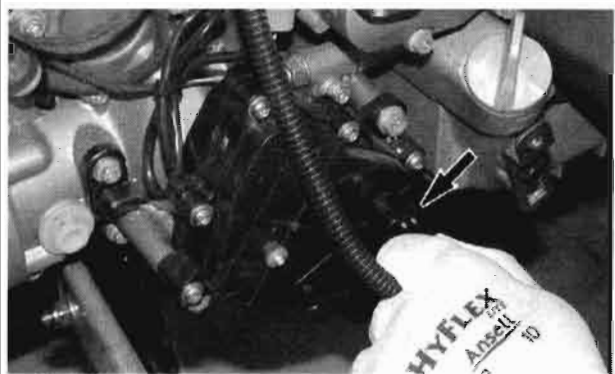
COUPLING UNIT CONNECTOR
