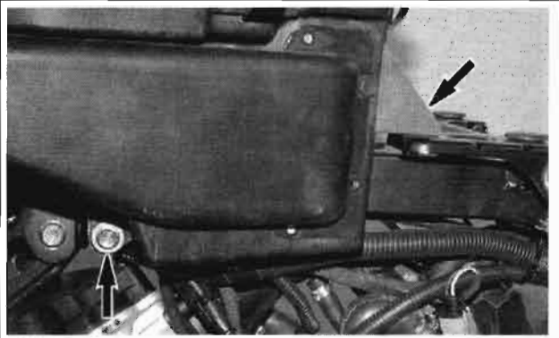
BOLTS RETAINING AIR FILTER HOUSING
