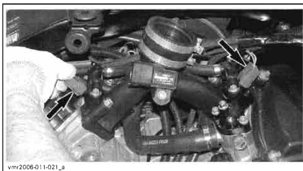
FUEL INJECTOR CONNECTORS
