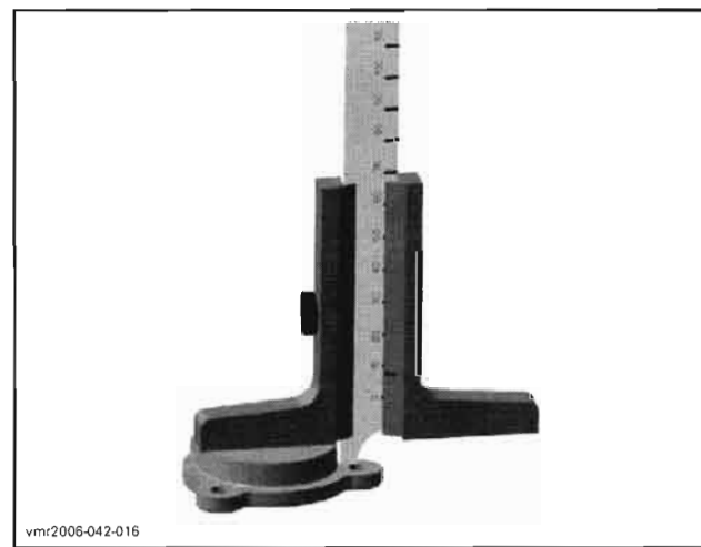
OIL PUMP COVER — MEASUREMENT "B"
